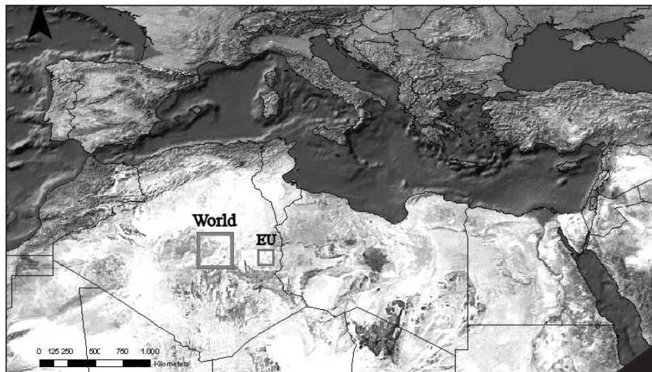
The larger square on the left shows a 254 km x 254 km area of hot desert that, if covered with concentrating solar power plants, would provide electricity equivalent to the current electricity consumption of the whole world. The smaller square shows a 110 km x 110 km area that would meet electricity demands of the European Union (when it included 25 countries).
